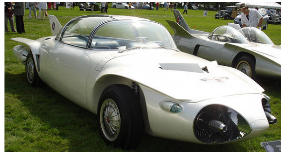
General Motors' Firebird II was described as having an "electronic brain" that allowed it to move into a lane with a metal conductor and follow it along.
