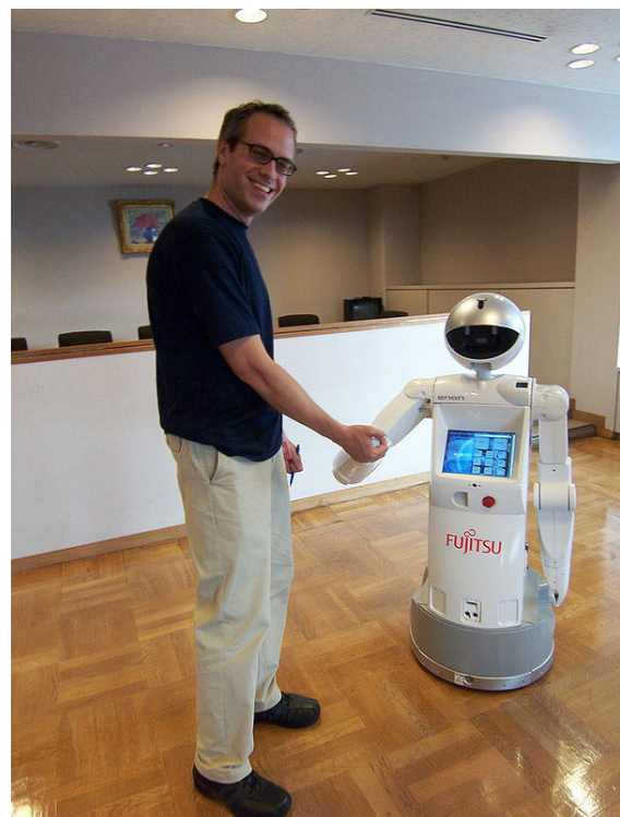
Enon was created to be a personal assistant. It is self-guiding and has limited speech recognition and synthesis. It can also carry things.
